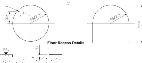
Concrete to BS 5328: 1997 specification, type ST5. Base to be flat and level to +/-5mm over footprint area. To level unit during installation use non-metallic shims only.
