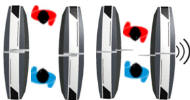
Wrong way direction/intrusion attempt
